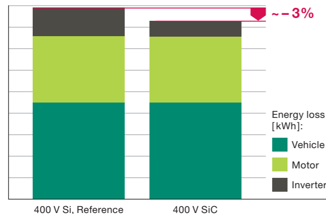
Figure 1: More efficient switching of a SiC compared to Si inverter at a voltage level of 400 V with same switching frequency (10 kHz) and voltage slew rate (5 kV/us).
