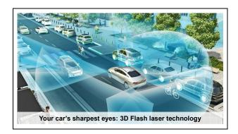
One of our drivers of growth is our pioneering laser technology. It will be ready for production by 2020. The technology incorporates a core optical system, which works using pulses of light, in a similar way to a series of flash photos. This provides an exceptionally accurate and distortion-free three-dimensional map of the vehicle's surroundings.
