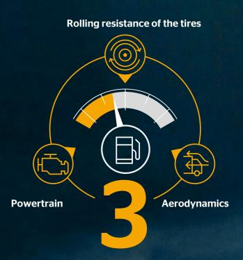
The level of CO<sub>2</sub> emissions is directly related to fuel consumption. The three main factors impacting on fuel consumption and CO<sub>2</sub> emissions are the drive system of a vehicle, its aerodynamics and the rolling resistance of its tires.
