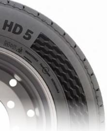
We recommend **replacing** tires once they are ten years old due to the increasingly advanced stage of the aging process. (Source: BRV)
