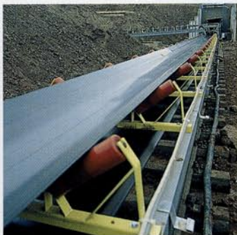
A brickmaking plant in Eastern Germany uses textile-ply belts to convey materials over a distance of 4½ miles.
