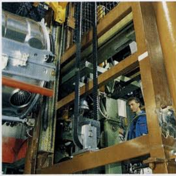
Large synchronous drive belts made from polyurethane are used in high-bay racking control systems.
