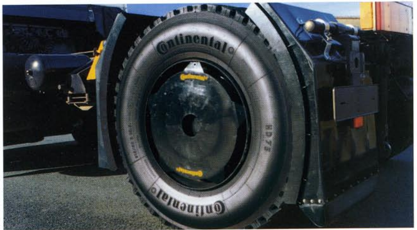
Wheel arches and wheel covers with integrated sound absorbers that are specially matched to the tires are a key segment of the Automotive Systems Group's business.
