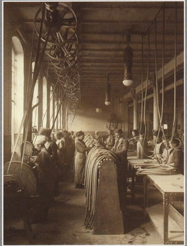
Finishing of bicycle tubes, 1921
