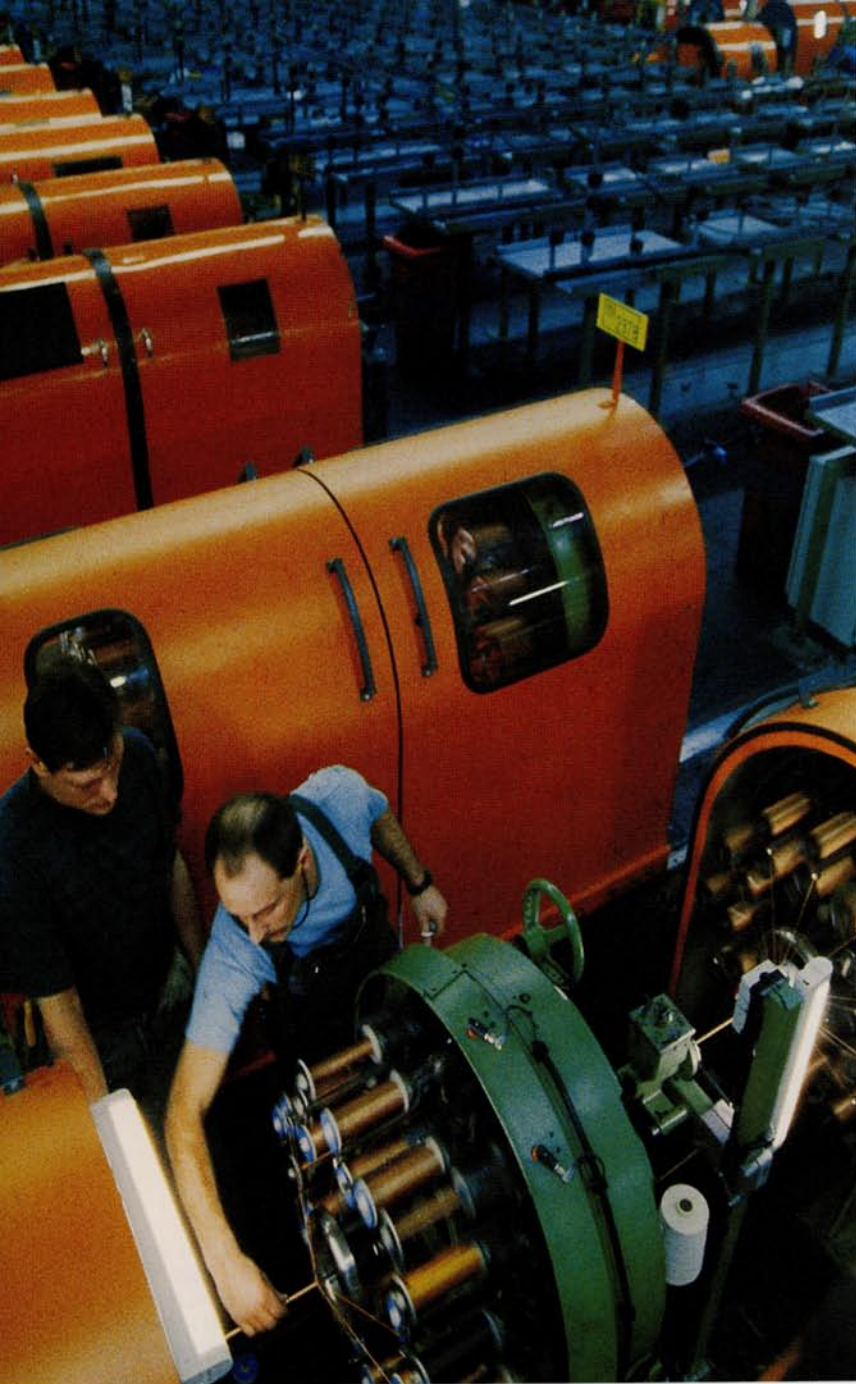
Modern bobbin machines are used in the production of hydraulic brake hoses.
