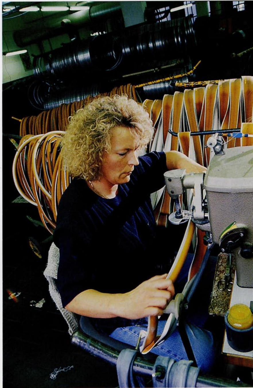
Meticulous needlework is essential when sewing tubes into performance tires for bicycle racing; gold medals may depend on it.
