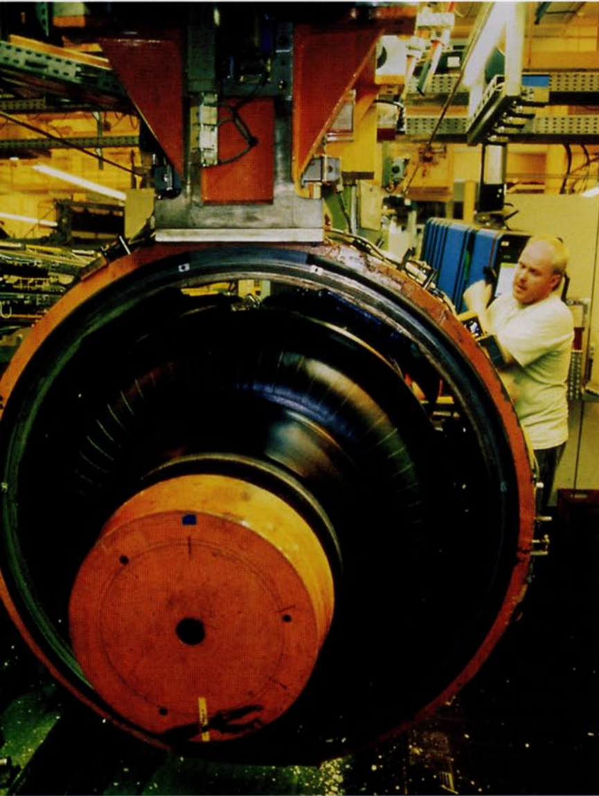
The carcass of a commercial vehicle tire is automatically joined to the tread/belt package by applying pressure and varying the tire's position.
