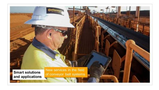
In ContiTech, we will achieve growth primarily with new, digital technologies. We use them to monitor conveyor belt systems. We also do this remotely with the help of drones, for example. The data is processed with artificial intelligence. In this way, we detect the condition of the belts and rollers with great precision. We can thus predict when there will be wear and tear. This allows our customers to better plan maintenance and repairs, saving them time and money.
