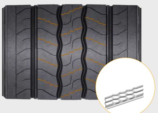
Full-width 3D matrix sipes deliver the right balance between flexibility and stability
