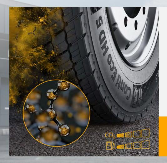
The tread package is the biggest contributor to overall rolling resistance. The new Eco Gen 5 combines an optimized tread compound with a new tire contour layout.
